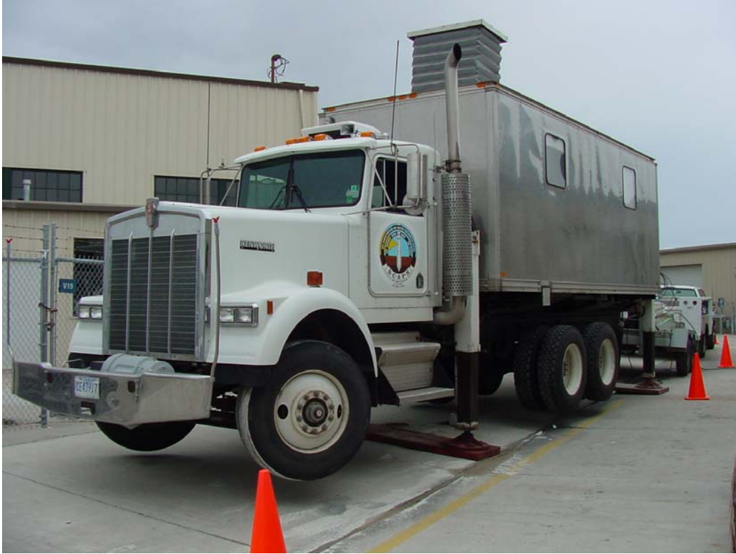
The SCAPS unit is drilling on the north end of Monterey Peninsula Airport to determine location and extent of contamination.
