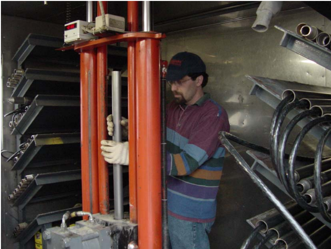
SCAPS crew member operating the Ram system inside the SCAPS truck.
