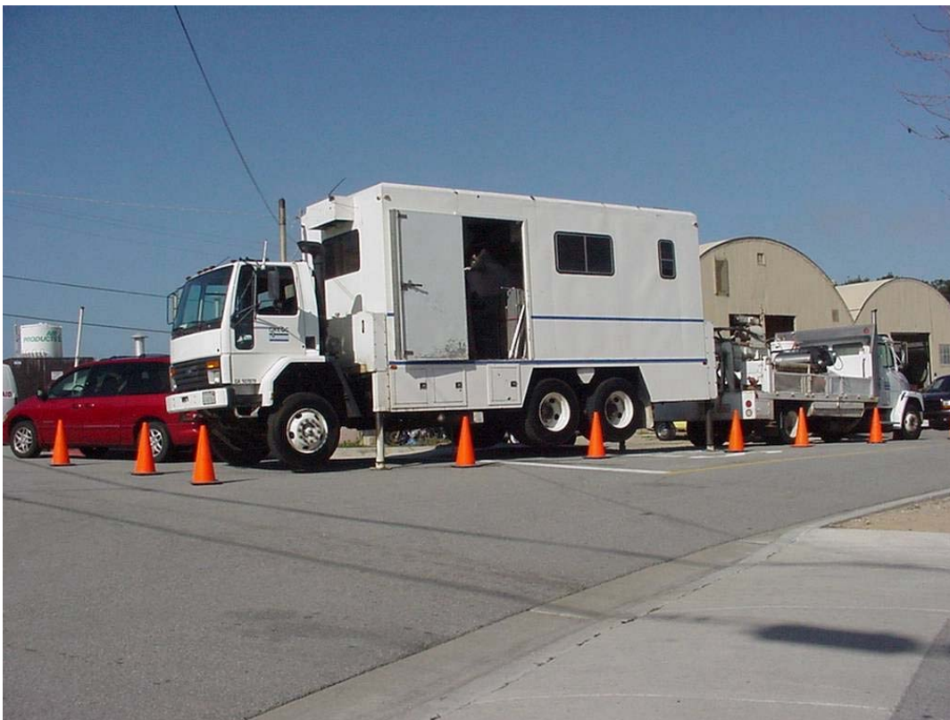
GREGG Drilling unit is taking samples near Quonset huts on airport property.
