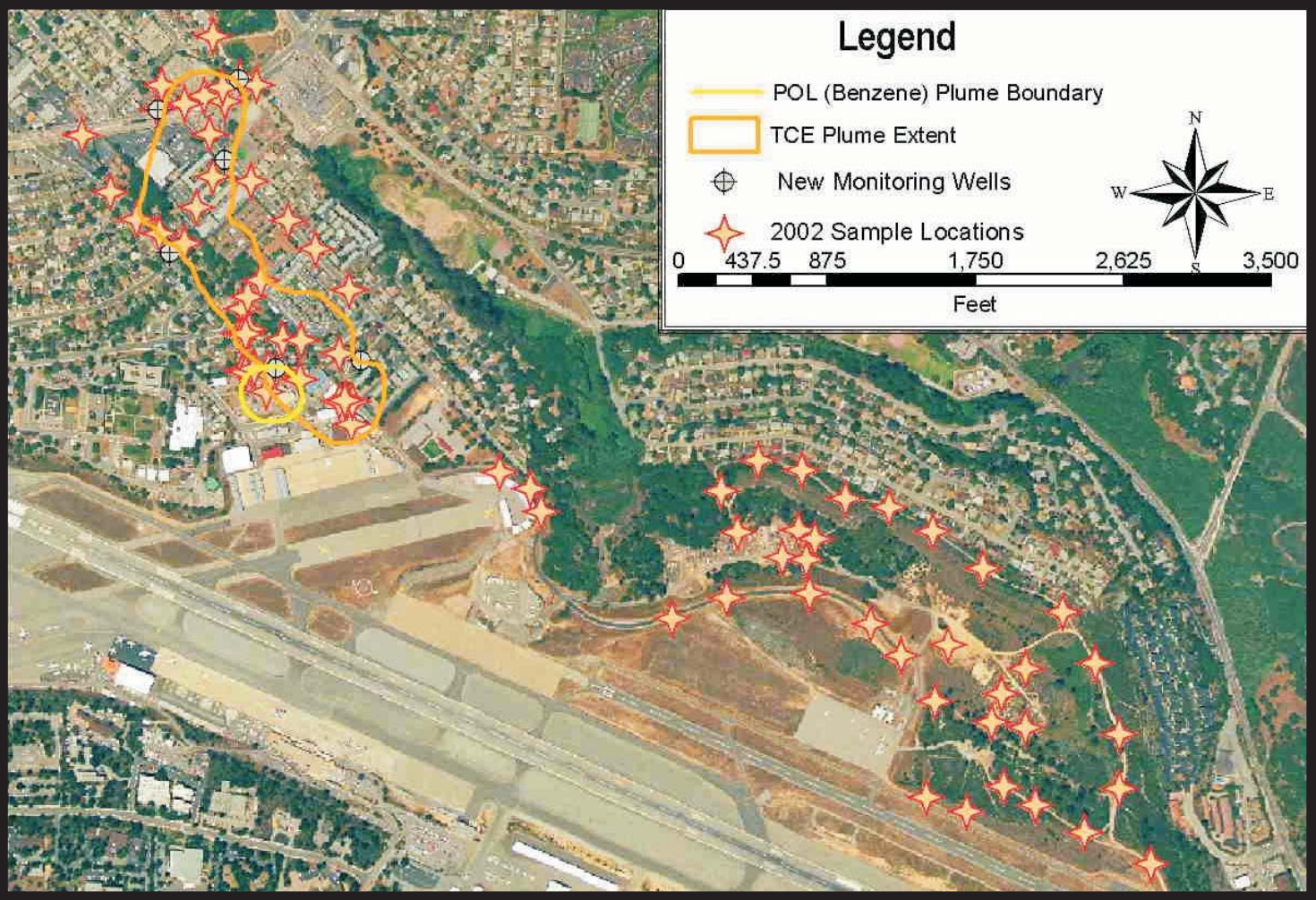
Sampling and monitoring well locations for the 2002 explorations plus newly defined boundary of the TCE plume.
